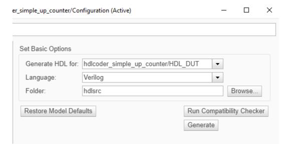
HDL Coder compiles the model before generating code. Depending on model display options such as port data types, the model can change in appearance after code generation. As code generation proceeds, HDL Coder displays progress messages in the MATLAB command line with links to the configuration set and the generated files. To view the files in the MATLAB Editor, click the links.
