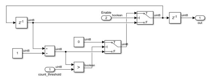
The Enable signal specifies whether the counter counts upward from the previous value. When the Enable signal is logical high, the counter counts up from zero to the count\_threshold value. When
