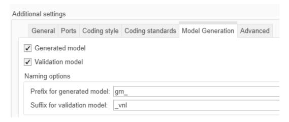
In the code generation logs, you see a link to the validation model. The validation model has the same prefix as the generated model and also has the suffix \_vnl. For the counter model, the validation
